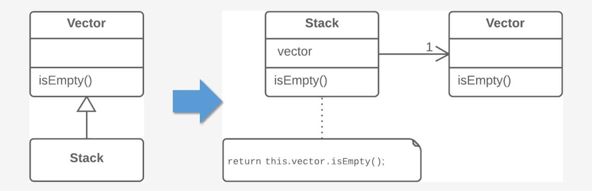
Create a field and put a superclass object in it, delegate methods to the superclass object, and get rid of inheritance.
